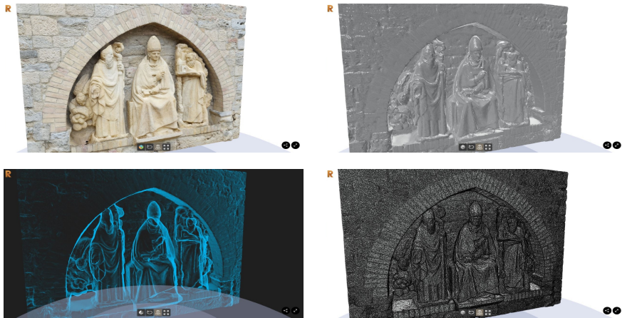
Figure 5.2: Four rendering possibilities provided by Autodesk ReMake [14]. In clockwise order starting from the upper left: textured, solid, wireframe, and X-ray mode. Interacting with the viewer controls, the final user can select in real time to visualize one of these options.
